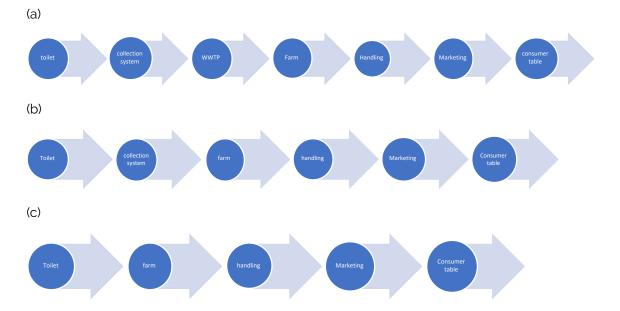
**Figure 1:** Control measures have to be established along the full sanitation chain whether a treatment plant is existing (a); a treatment plant is not existing (b); neither treatment plant nor collection system is existing.
